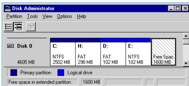
The figure shows a system with two primary partitions (C:(NTFS) and H:(FAT)) and one extended partition having two logical drives (D: (FAT) and E:(NTFS))
