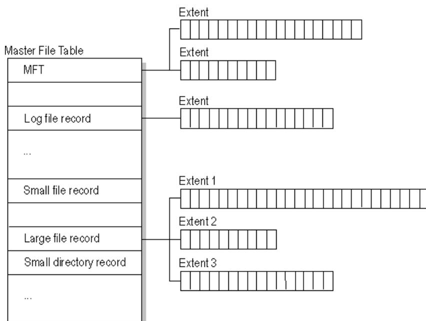
**Figure 32: Simplified illustration of the MFT structure**
