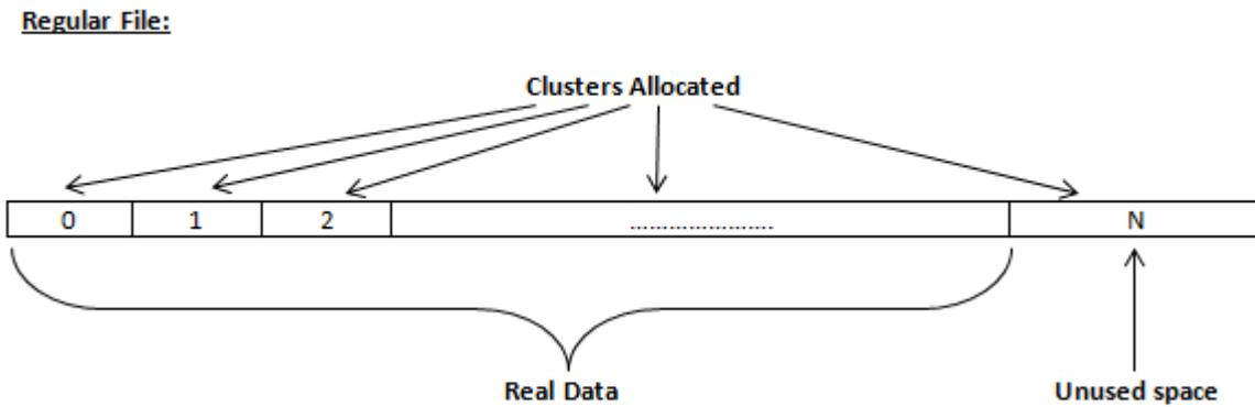
**Figure 38: File Slack Space and Allocated Clusters**
