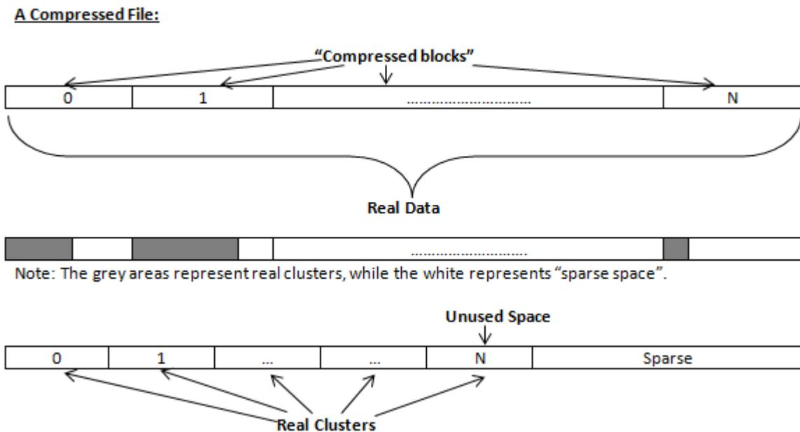
**Figure 39: Compressed File Structure**
