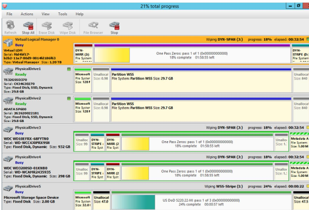
**Figure 30: Erasing a Virtual Drive (Striped Disk Array)**
