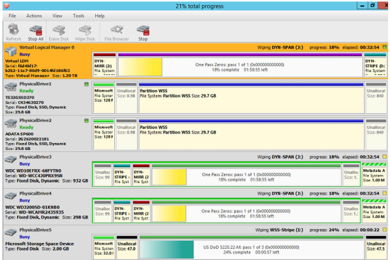
**Figure 47: Erasing a Virtual Drive (Striped Disk Array)**
