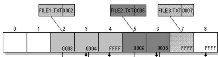
**Figure 35: Example of File Allocation Table**
